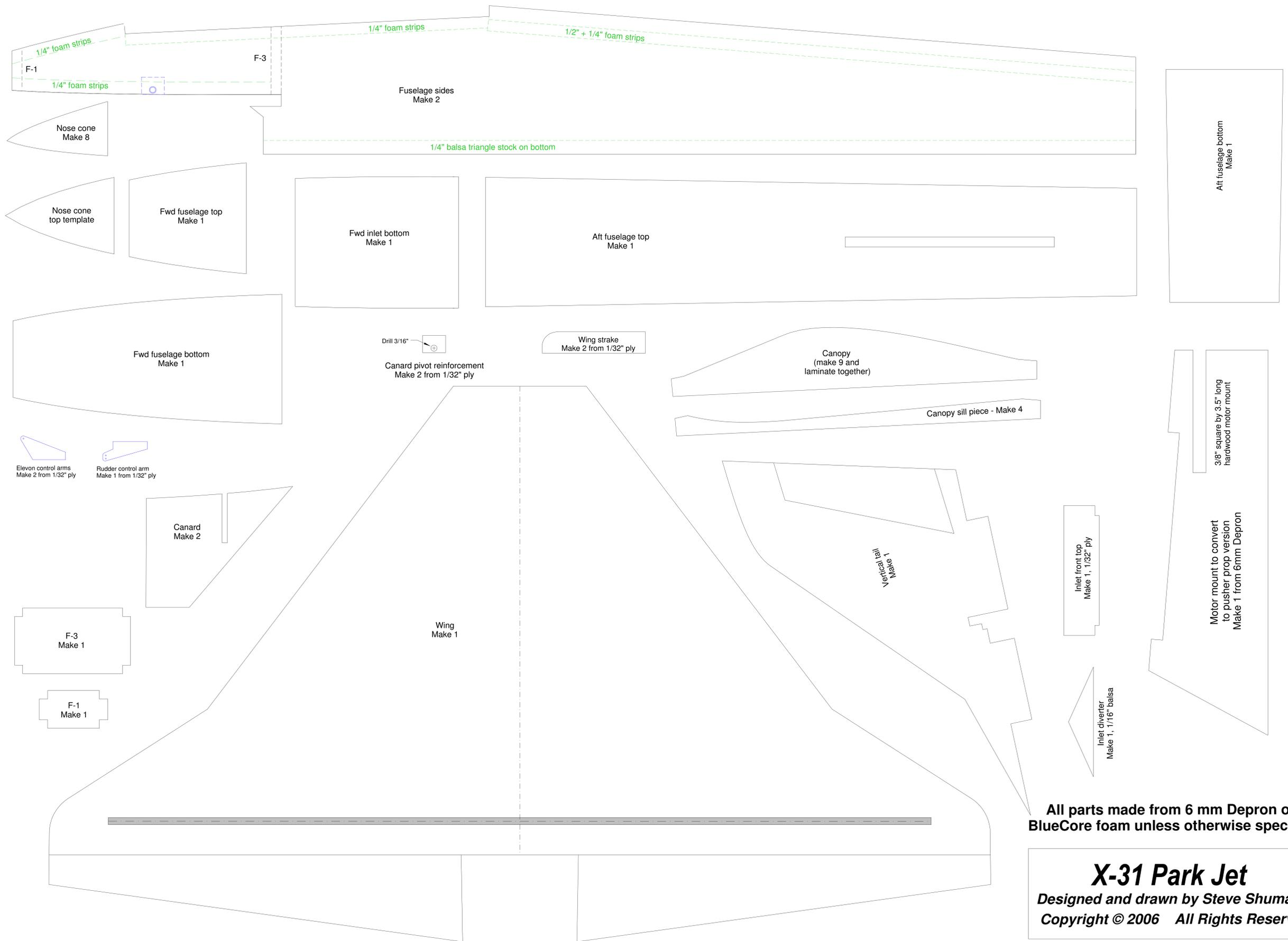
All parts made from 6 mm Depron or BlueCore foam unless otherwise specified
