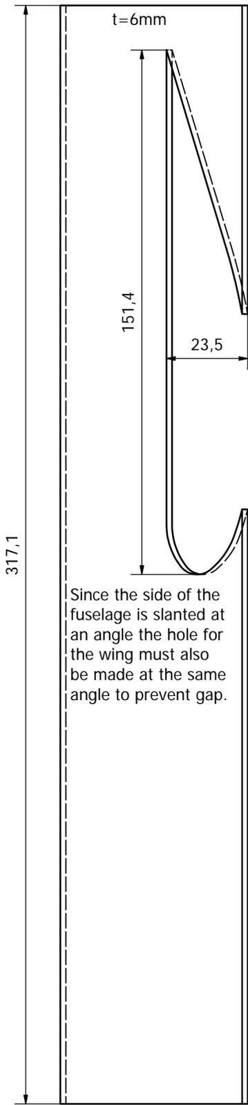
Since the side of the fuselage is slanted at an angle the hole for the wing must also be made at the same angle to prevent gap.
