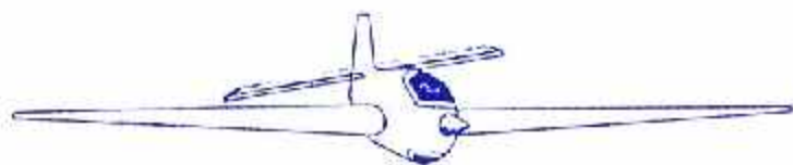
Fig. 3 In left rudder knife edge the top of the stab can be seen (i.e. positive pitch).
