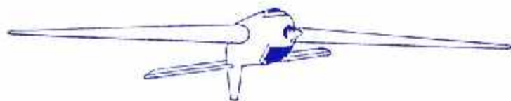
Fig. 4 In right rudder knife edge the bottom of the stab can be seen (i.e. negative pitch).
